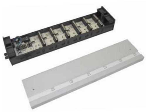
Terminal block enables connection of thermostats and servomotors in one place (e.g. in a cabinet over the manifold). It is possible to connect max. 6 thermostats and 12 servomotors.
