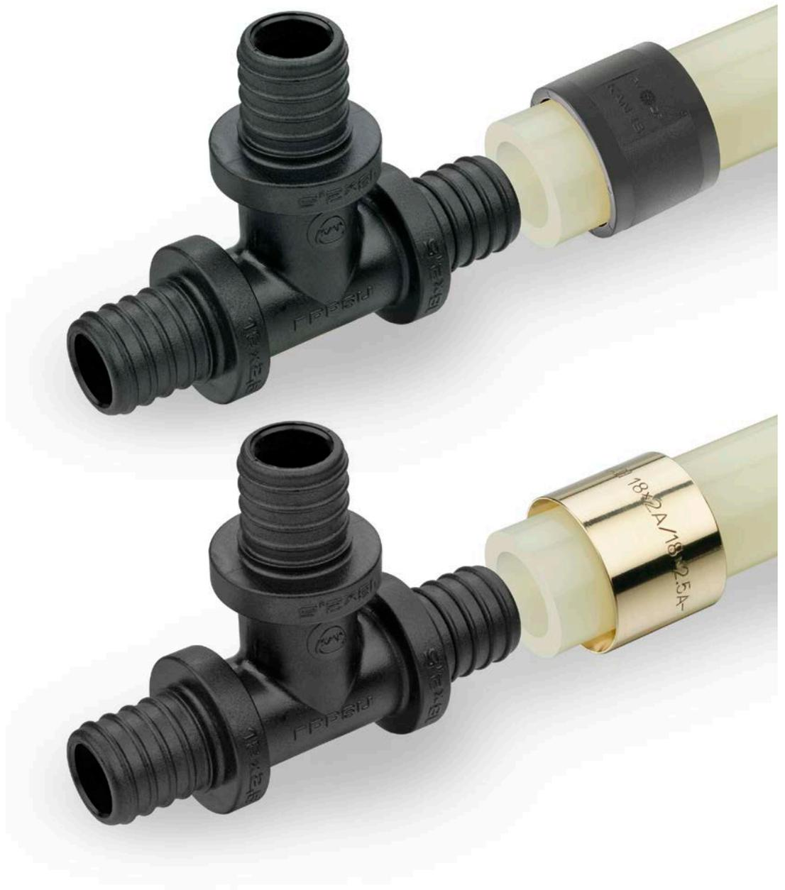
A KAN-therm Push System leak-tight joints without O-Rings are made by pushing a brass sleeve onto a fitting and a pipe. These joints do not require additional sealing like a PTFE tape or tow. Other complementing elements of the system are manifolds and installation cabinets.
