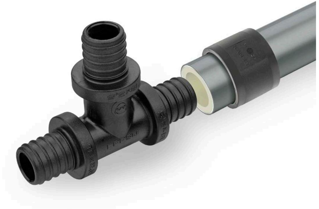
Push Platinum System leak-tight joints without O-Rings are made by pushing a brass sleeve onto a fitting and a pipe. These connections do not require additional sealing like a PTFE tape or tow. The system is complemented by manifolds and installation cabinets available in section Manifolds, cabinets and accessories.
