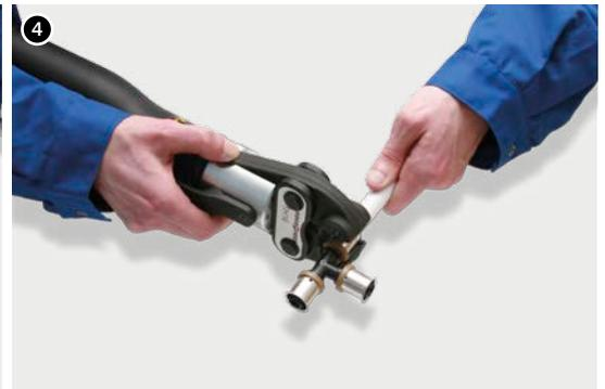
4. Apply the press jaws exactly on the steel ring between the plastic distance ring and the steel ring collar perpendicularly to its axis. In case of the "TH" profile place the jaws on the plastic distance ring (the ring must be embraced by the jaws outer groove). In both cases due to the fitting design the clamping tool jaws will not shift during pressing.
