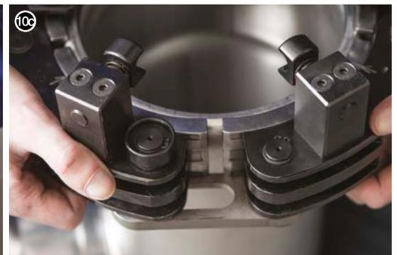
The unfolded jaw is put onto the fitting. The press jaw has a groove which should fit the flange fittings. After correct fitting the jaw on the fitting you should secure it by pressing the pin again and locking the adapter.
