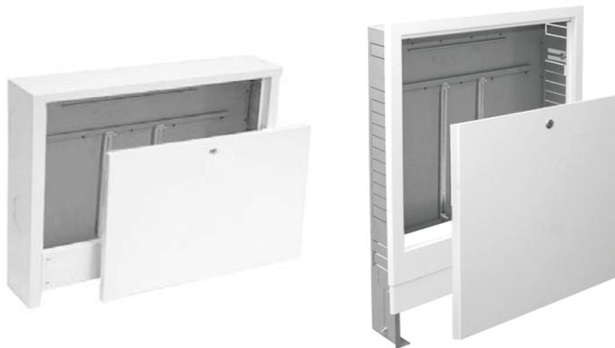
Due to the design of cabinets for floor heating manifolds can be mounted with or without a mixing device. In cabinets there is also room for electrical terminal blocks. Terminal blocks are attached by screws, which enter into special holes in a mounting strip in the upper part of a box.
