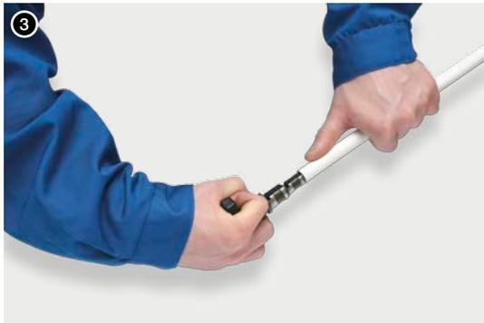
4. Insert the screwed joint body into a pipe till it definitely stops. The joint insertion depth is ca. 9 mm for pipes Ø14, 16, 20 and 12 mm for pipes Ø25, 26.
