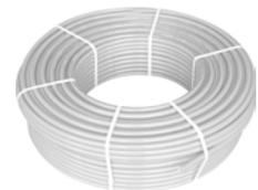
Operating parameters  $T_{work}$  90°C ( $T_{max}$  - maximum 95°C,  $T_{mal}$  - malfunction 100°C), pressure 10 bar, for central heating and underfloor heating systems.
