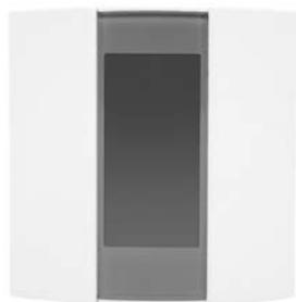
**230V weekly thermostat with floor sensor** - allows for individual adjustment of temperature in the room. The thermostat has the function of weekly programming. It is equipped with a floor temperature sensor. The thermostat has the option of a manual and automatic control. It may cooperate with Basic and Basic+ terminal blocks in 230V version.
