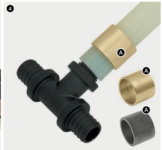
**4.** Insert the fitting into a pipe up to the last bead on the fitting.
