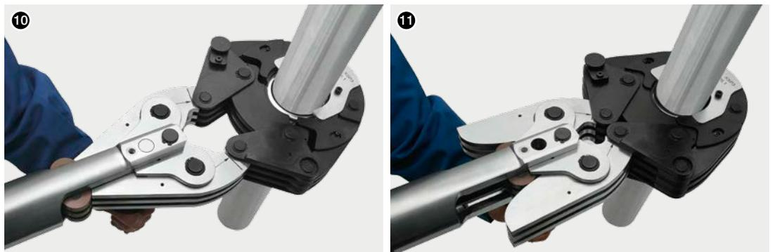
10 **Assembling the machine to the jaw**
