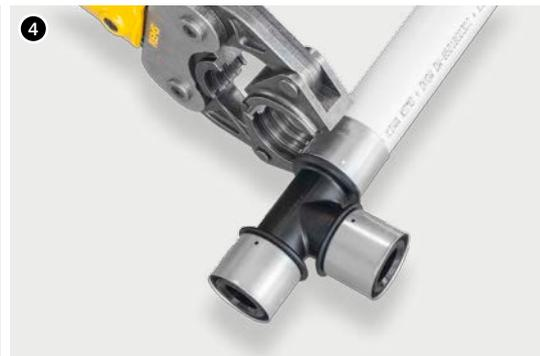
5. Apply the clamping tool jaws on a ring so it contacts the tube coupling collar. The external collar of jaws shall be pushed to the tube coupling collar but not embrace it. Start the clamping tool drive and make the connection.
