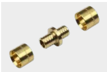
Slika 49. KAN-therm Push spojke (fitingi) za cevi PEXC, PERT in bluePERT, premeri 12 × 2, 14 × 2, 18 × 2, 18 × 2,5, 25 × 3,5 mm.
