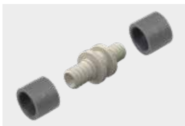
Slika 50. Spojka (fiting) KAN-therm ultraLINE za cevi PEXC, PERT 2 in PERTAL 2 , premeri 14 × 2, 16 × 2,2, 20 × 2,8, 25 × 2,5 mm.
